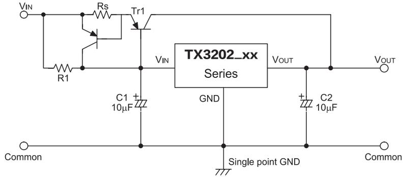
Circuit for Increasing Output Voltage
