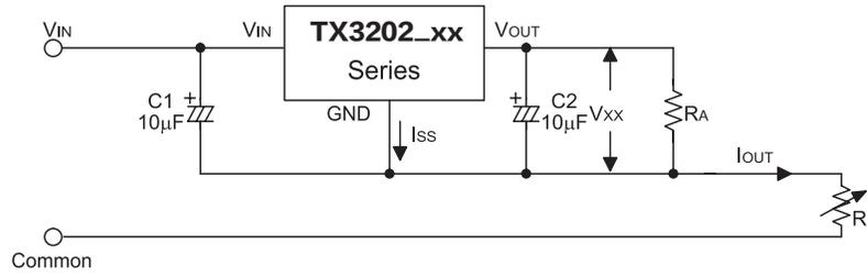
$$I_{OUT} = \frac{V_{XX}}{R_A} + I_{SS}$$
