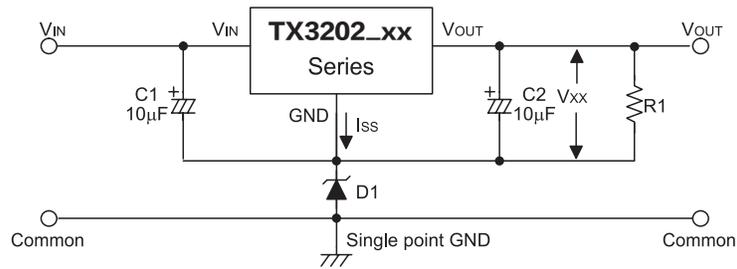
$$V_{OUT} = V_{xx} + V_{D1}$$
